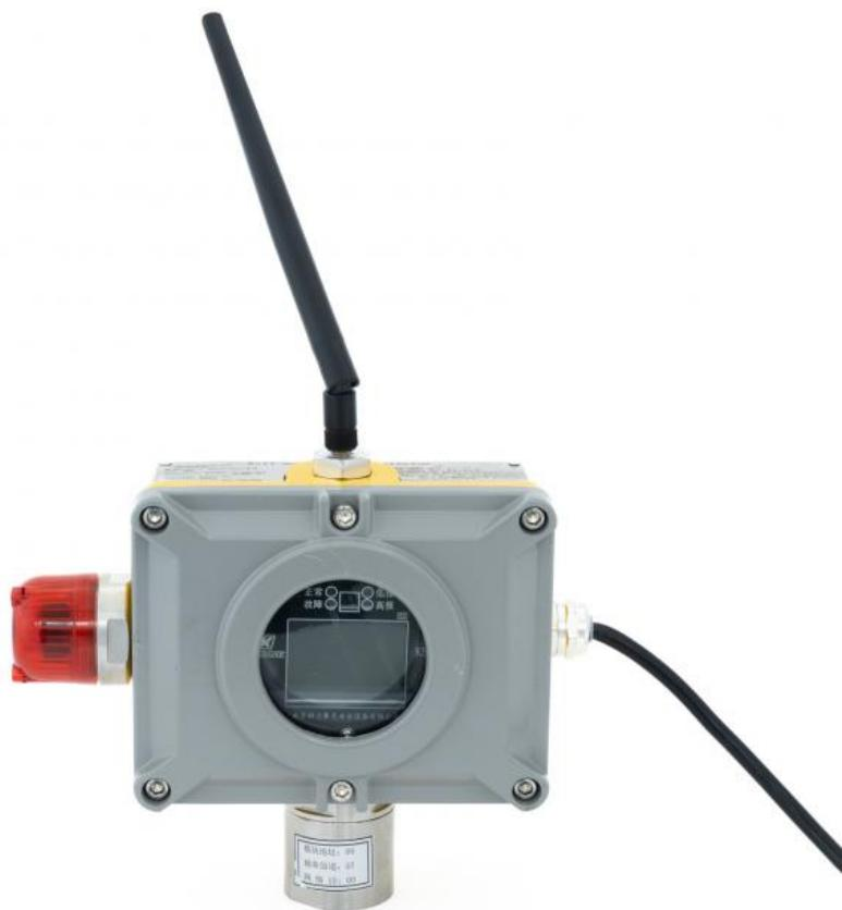
**The K500 series wall-mounted gas detector**, made with imported high sensitivity sensors and an explosion proof design, has a long service life. This wall mounted gas detector works as part of an integrated system (with 4-20 mA analog output) or only as an independent system. It has two alarm levels (high level & low level), with different audible and visual alarm signals.
