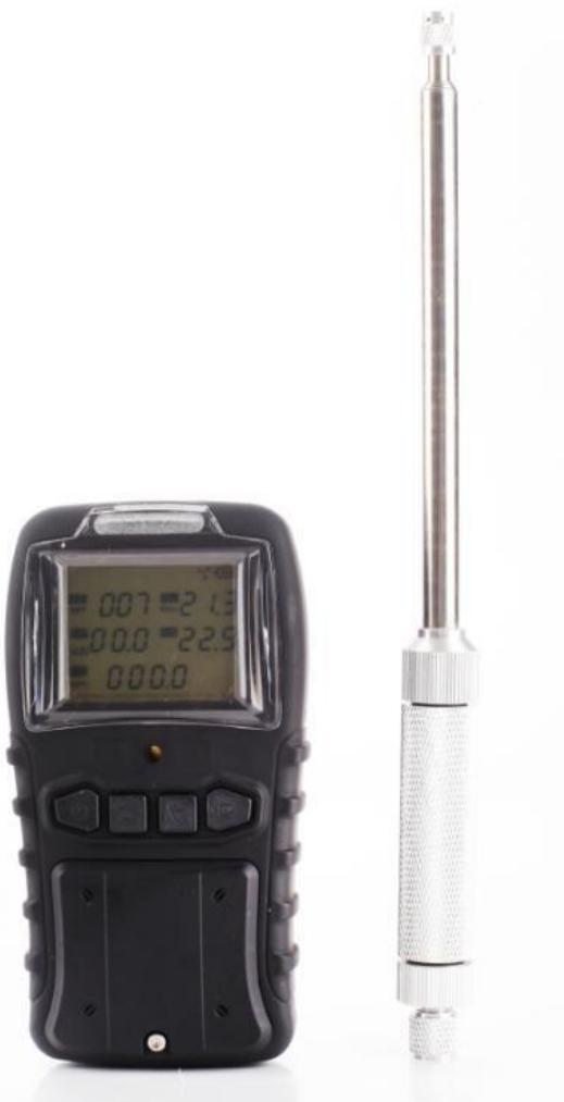
The K60-V is a full-featured, compact, up to five sensor gas detector for oxygen, combustibles, hydrogen sulfide, carbon monoxide, sulfur dioxide or VOCs etc (gas types could be optional customized based on clients' requests). Key features include easy-to-operate design, easy-to-identify color screen 4 digits LCD display, history data storage, a water-resistance case and high sensitivity sensors.
