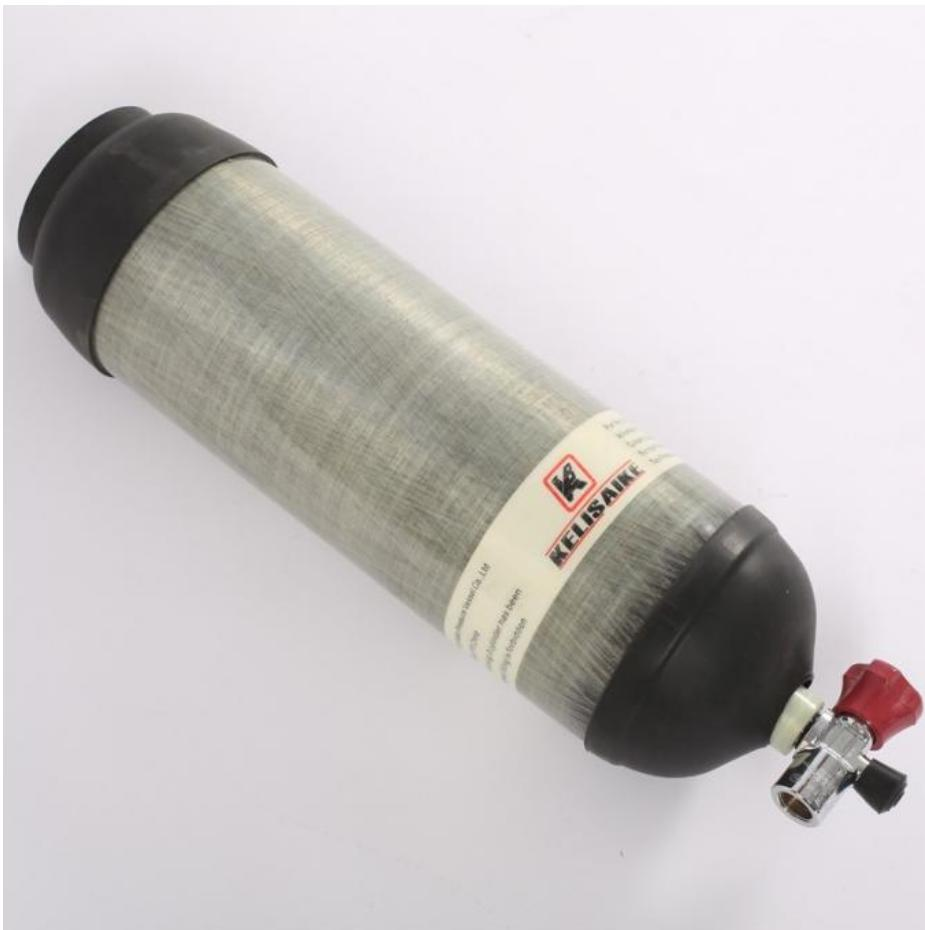
Y shape design, with safe self lock device to prevent inadvertent close due to hard knock or incorrect operation. Unscrew the switch handwheel by rotating in the counterclockwise direction, it is regarded as the open condition and close vice versa. There is safety diaphragm set in cylinder valve, with explosion pressure at(37-45)Mpa to prevent the deformation and explosion of cylinder due to inner high pressure.
