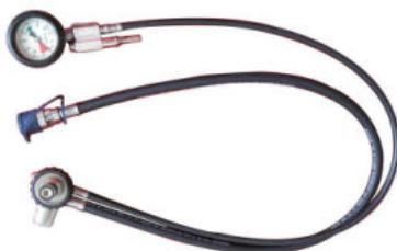
The warning whistle is integrated with pressure gauge and located on the chest after donning. It will give a continuous 90dB alarm to make sure the user can hear it under noisy environment.
