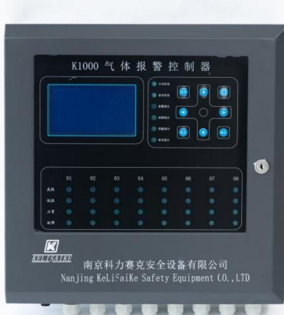
K1000 series gas detector controller provides simultaneous display and alarm functions for up to 4 or 8 or 16 monitored variables. Easy to configure and user friendly, the K1000 series control system can function as a critical alarm controller for toxic or combustible gases. The controllers are easy to install and feature a large graphical LCD display and non-intrusive user interface for hazardous areas.
