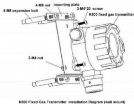
K800 Fixed Gas Transmitter Installation Diagram (wall mount)
