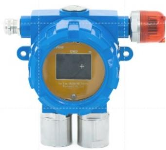
K900 fixed gas detection transmitter can be widely used in metallurgy, petroleum, petrochemical, chemical, shipbuilding and other industries. The instrument adopts explosion-proof design, (4 ~ 20) MA standard signal output, which can be transmitted remotely and directly into DCS system. The detection sensor has the characteristics of high sensitivity, rapid response, long service life and short polarization time, and is at the leading level of similar products in China.
