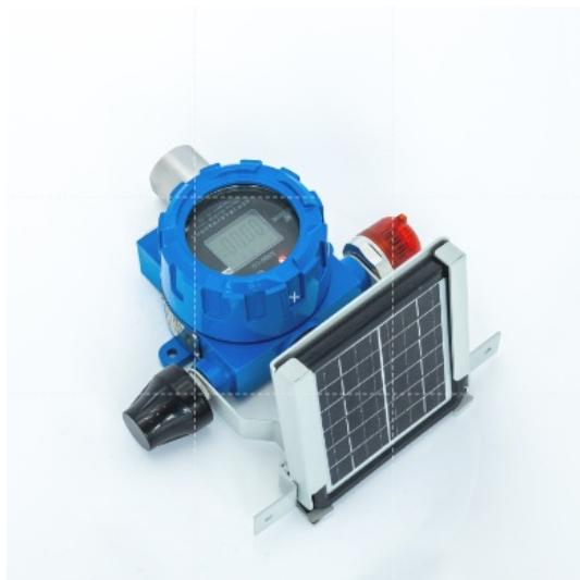
K900 fixed gas detection transmitter can be widely used in metallurgy, petroleum, petrochemical, chemical, shipbuilding and other industries. The instrument adopts explosion-proof design,(4 ~ 20) MA standard signal output, which can be transmitted remotely and directly into DCS system. The detection sensor has the characteristics of high sensitivity, rapid response, long service life and short polarization time, and is at the leading level of similar products in China.
