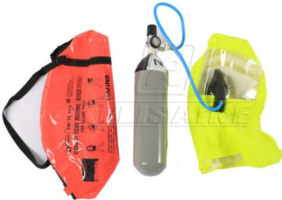
This product has successfully obtained **CCS certification** and holds the official ship inspection certificate, ensuring compliance with stringent maritime safety standards. The emergency escape breathing device is composed of several key components: a compressed air cylinder, pressure reducer, pressure gauge, gas conduit, protective hood, backpack harness, and related accessories.
