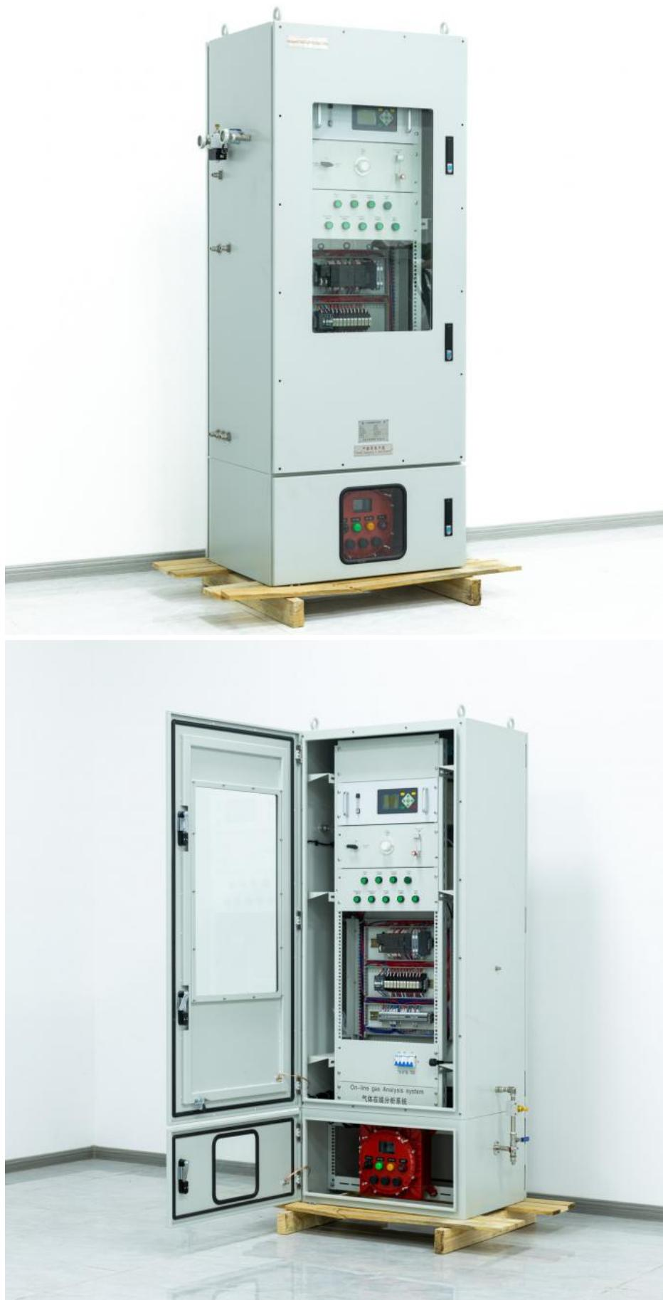
The KELISAIKE SAFETY CEMS is designed for real-time, automated monitoring of flue gas composition and related parameters. It is capable of measuring **SO<sub>2</sub>, NO, CO, O<sub>2</sub>, dust concentration, as well as flue gas flow, pressure, and temperature**. The system can be configured and optimized according to the specific site conditions and technical requirements, enabling precise measurement of gaseous pollutants and particulates for effective quantitative control of
