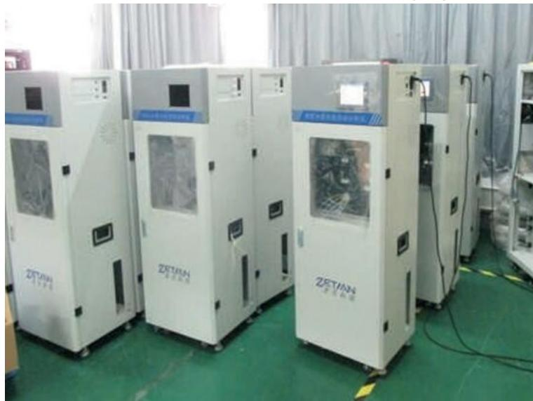
The analyzer based on UV absorption spectroscopy and chemometric algorithms to measure SO<sub>2</sub>, NO<sub>x</sub>, O<sub>2</sub>, NH<sub>3</sub>, Cl<sub>2</sub>, O<sub>3</sub>, H<sub>2</sub>S and other gases concentration,
